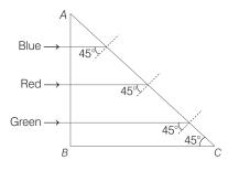
At face AB, i = 0. So, r = 0, *i.e.*, light will be incident on face AC at an angle of incidence  $45^{\circ}$ .
